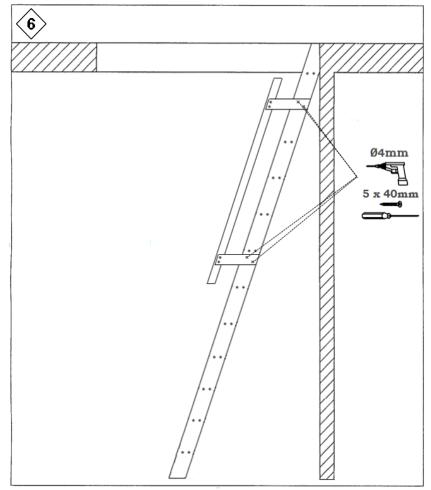
The handrail comes pre-assembled ready for you to fit to the ladder. Once you have decided on its position then drill through the pre-holed handrail into the string to create your pilot holes. You can then screw the handrail to the string with the 5 x 40mm screws provided.
