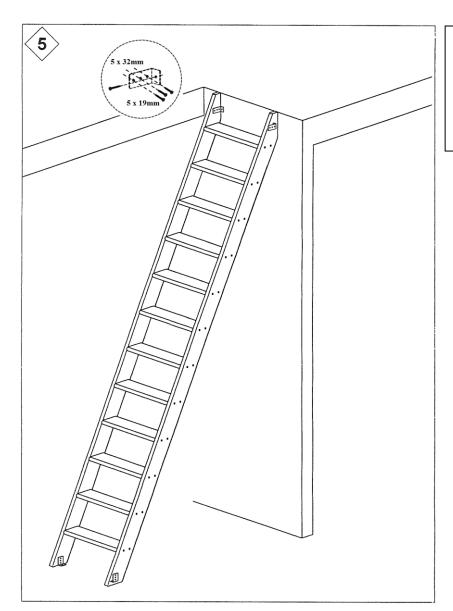
The top of the ladder strings come square so if fitting against a wall then the strings can be cut (as picture 5). When fixing the brackets at the top and bottom of the ladder, pilot holes will need to be made in the strings making it easier to screw the brackets to them.
