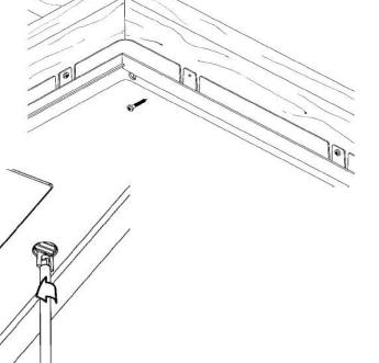
**5.** Finally replace the door into the frame ensuring both hinge lugs are correctly located. Secure door by turning catch anti-clockwise. This can be done using a pole (not supplied) with the pole end (supplied).
