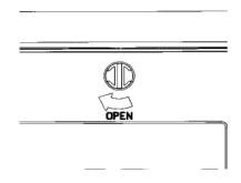
**2.** Swing the door open as far as it will go and then slide side ways slightly to disengage one side of the hinge then remove the door.
