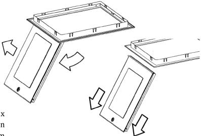
**3.** Trim out a suitable opening 562 x 726mm. Locate frame into position pushing tightly against the ceiling to form seal.
