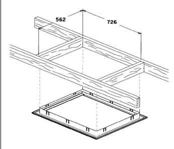
**4.** Screw through the fixing points in ten places as shown. Note suitable packing pieces may be required if the opening is over size, to prevent the distortion of the frame.
