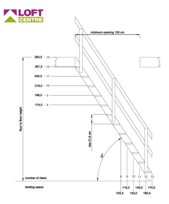
To establish the amount of floor space (Going) the **Lisbon** Staircase will take up all depends on your Floor to Floor height. By looking at the above diagram will give you a guide to the floor space (Going) that will be required. For Example if your Floor height is "2400mm" then the **Lisbon** Staircase needs to be altered to 11 Risers. The Going for 11 Risers is "1460mm" indicated at the bottom of the diagram.
