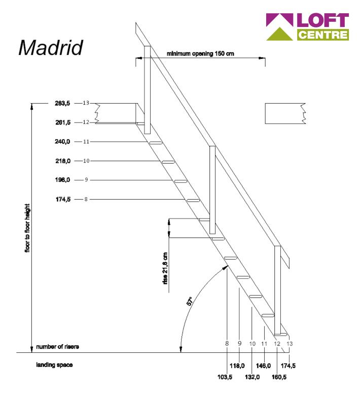
To establish the amount of floor space (Going) the **Madrid** (**Miller**) Staircase will take up all depends on your Floor to Floor height. By looking at the above diagram will give you a guide to the floor space (Going) that will be required. For Example if your Floor height is "2400mm" then the **Madrid** Staircase needs to be altered to 11 Risers. The Going for 11 Risers is "1460mm" indicated at the bottom of the diagram.
