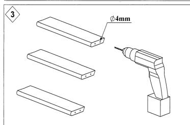
The treads will require pilot holes ready to take the screws. This is done by positioning the tread into the string (#) then drilling through the pre-holed string into the tread to create your pilot hole. Two pilot holes in both sides of the treads will be needed (as image above).
