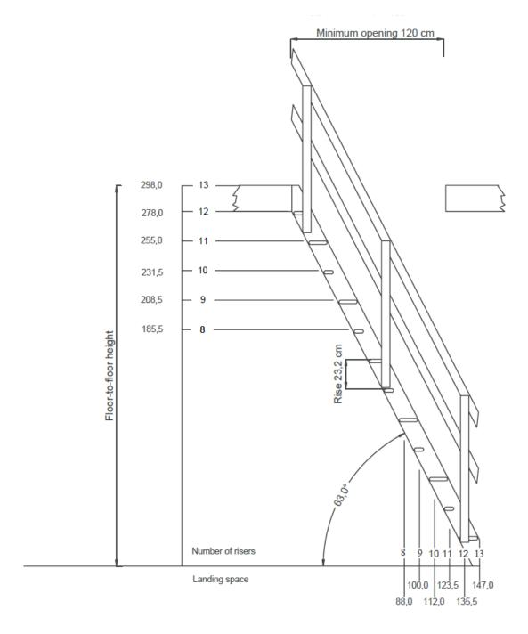
To establish the amount of floor space (Going) the **Amsterdam** Staircase will take up all depends on your Floor to Floor height. By looking at the above diagram will give you a guide to the floor space (Going) that will be required. For Example if your Floor height is "2550mm" then the **Amsterdam** Staircase needs to be altered to 11 Risers. The Going for 11 Risers is "1235mm" indicated at the bottom of the diagram.
