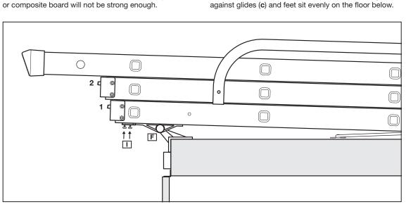
17. Release the lock catch on the top ladder section (1) and slide the middle section up until it locks. Release the lock on the middle section (2) and slide the bottom section up until it locks. Use the pole to fully stow the ladder. With the ladder fully stowed, slide the retainers
