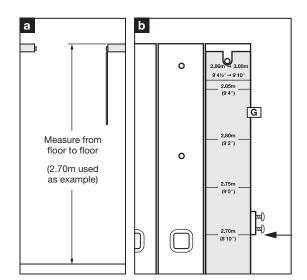
**10.** Measure the distance between the floor of the room to the floor of the loft (2.70m used as example) (a). Place paper template (G) on back ladder section with the cutout lining up with the top hole. Position the stop at the required height (2.70m used as example), tighten both stop screws (b). Repeat with stop on other side of ladder.
