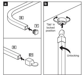
**5.** Fit the ends to the pole (a). **To lock:** Turn anticlockwise, **To unlock:** Turn clockwise (b).
