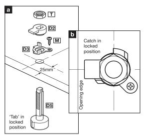
**3.** Assemble the catch. Assemble the catch onto the trapdoor ensuring the 'tab' on the catch barrel and the catch are positioned as shown (a). **Note:** Only fix the retaining washer (**D3**) using the 12mm screw (**M**) once correctly positioned as shown above (b).
