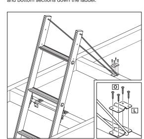
**16.** Attach the pivot arm to the loft floor/wooden batten (this may have to be added at the correct distance) using the pivot arm bracket. Use a bradawl or small drill to start the screw holes, attach the bracket (**L**) to the loft floor using 4 x 20mm screws (**O**).
