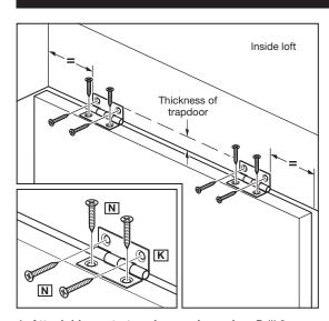
1. Attach hinges to trapdoor and opening. Drill 2mm pilot holes, attach hinges (K) to trapdoor and surround using 8 x csk 20mm screws (N). Note: The trapdoor will attach to the same side of the opening as the ladder (Trapdoor is not supplied).
