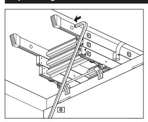
**18.** To lower ladder. Insert the pole (B) into the round hole on the bottom ladder section and carefully pull down until bottom section rests on top stops.
