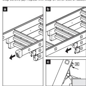
14. Fully extend ladder out of loft opening. Release the lock catch on middle ladder section and extend bottom section until it locks (a). Repeat with the catch on the top section and extend the middle section until it locks (b). Important: Ensure top stops (H) are tight against glides (c) and feet sit evenly on the floor below.
