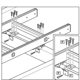
**13.** Ensure both pivots (**F**) are spaced as far apart as possible (up against the glides). Use a bradawl or small drill to start the screw holes, attach the pivots to the trapdoor surround using 10 x 25mm screws (**P**). **Note:** The trapdoor surround must be solid wood. Chipboard
