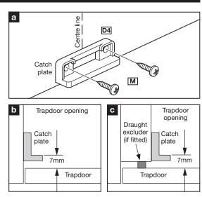
**4.** Attach catch plate. Find and mark the centre line onto the opening end of the trapdoor surround. Allow a 7mm gap between the top of the catch plate and the trapdoor (**b** or **c**). Attach the catch plate (**D4**) to the trapdoor surround using 2 x 12mm screws (**a**).
