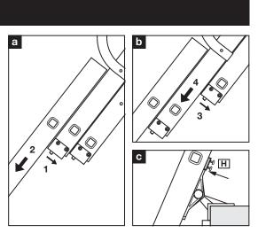
19. When ladder comes to a stop, release catch on middle section (1) and lower bottom section (2) until it locks into place (a). Release catch on top section (3) and lower middle section (4) until it locks into place (b). Important: Ensure top stops (H) are tight against glides (c) and feet sit evenly on the floor. To stow ladder repeat steps 18 and 19 in reverse order.
