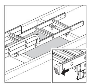
**12.** Using a suitable ladder gain access to the loft and position the ladder centrally across the loft opening with the pivot assembly resting squarely on the trapdoor surround. To help with access, release the lock catch on the end of the top ladder section and slide the middle and bottom sections down the ladder.
