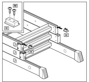
**7.** Loosely insert 12mm screws (**M**) into both stops (**H**) and slide into the top ladder section.
