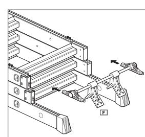
8. Slide the glide/pivot assembly (F) into the ladder, ensure it is fitted the correct way around as shown.
